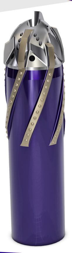
The REAPER reamer shoe has been specifically designed to be an aggressive shoe for extreme wellbore conditions. The nose is designed to aid in getting casing to T.D. by using coated blades and optimized jetting to ream and clean out the hole as casing is run. The body blades have tungsten carbide buttons to further assist with hole cleaning.
