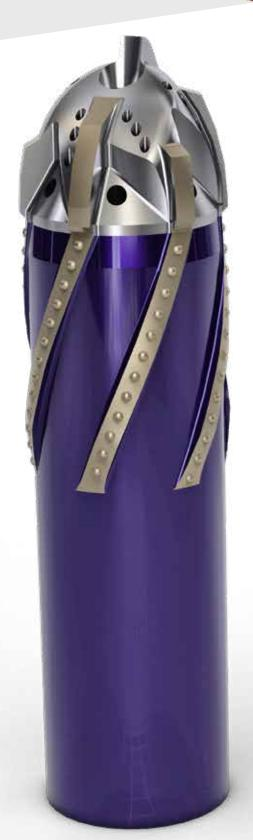
The Reaper reamer shoe has been specifically designed to be an aggressive shoe for extreme wellbore conditions. The nose is designed to aid in getting casing to T.D. by using coated blades and optimized jetting to ream and clean out the hole as casing is run. The body blades have tungsten carbide buttons to further assist with hole cleaning.
