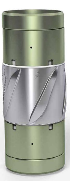
The CaseRUNNER Advanced Casing Drilling Centralizer, is an engineered torque reducing centralizer designed specifically for the casing drilling / liner drilling market. Utilizing proven friction reducing materials, the CaseRUNNER minimizes torque and vibration while casing drilling by centralizing the casing string and providing an 'ultra low friction' bearing surface, enabling smooth rotation of the casing.
