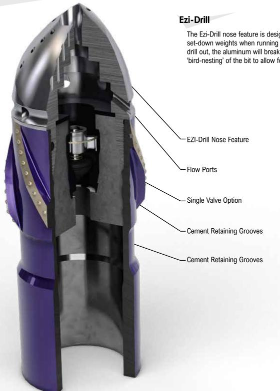
The Ezi-Drill nose feature is designed to withstand high set-down weights when running the casing to T.D. during drill out, the aluminum will break into small chips to avoid 'bird-nesting' of the bit to allow for a quick drill-out time
