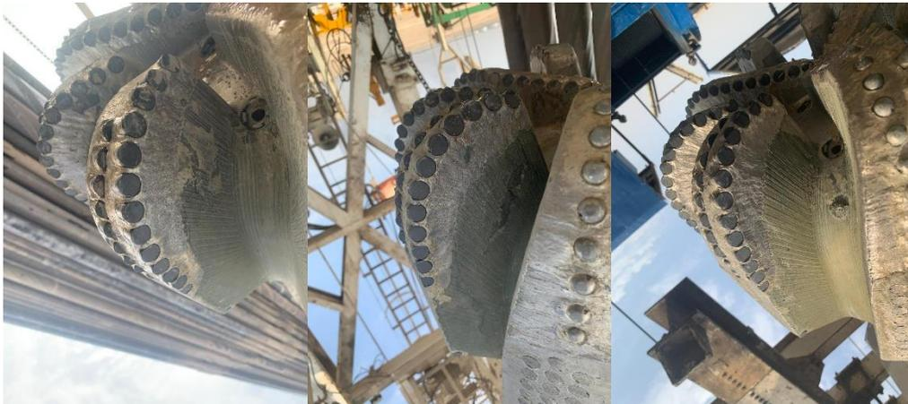
Fig. 17 – 22” PDC Bit picture after RSS run
