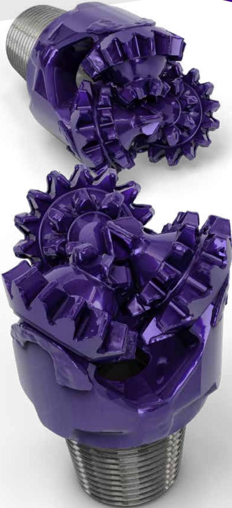
Varel's classic open bearing steel teeth bits for remedial, re-entry, and water well applications. All bits incorporate open throat hydraulics and can accommodate either regular through string flow or reverse circulation which is frequently used to re-enter wells. L2, L1, and LH1 are offered from softest to hardest of the cutting structure applications.
