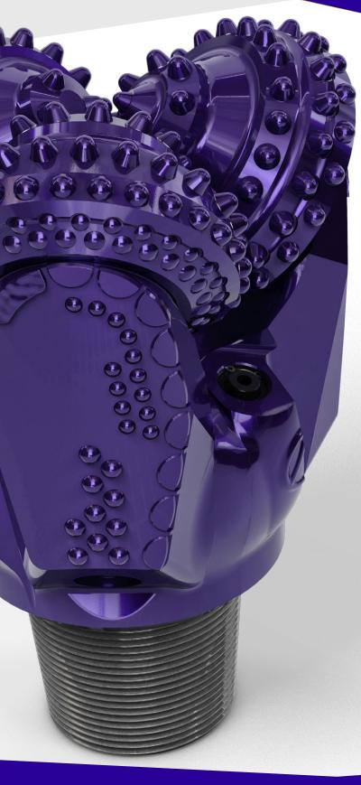
Sealed journal bearing air bits meet the need of air, water mist, and foam fluid systems to drill in all under-balanced applications. A-FORCE TCI cutting structures are specifically designed for use in underbalanced drilling regardless of the fluid system being utilized. A sealed journal bearing system improves bearing heat management and accommodates increased drilling parameters.
