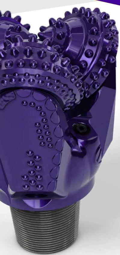
Sealed journal bearing air bits meet the need of air, water mist, and foam fluid systems to drill in all under-balanced applications. A-FORCE TCI cutting structures are specifically designed for use in underbalanced drilling regardless of the fluid system being utilized. A sealed journal bearing system improves bearing heat management and accommodates increased drilling parameters.
