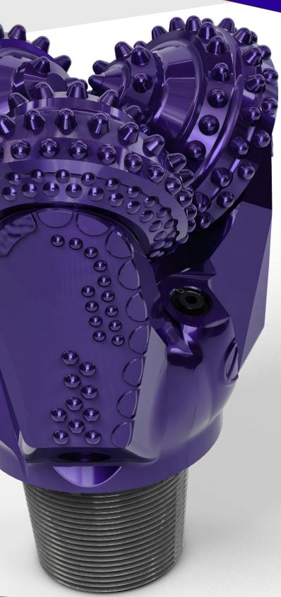
Sealed journal bearing air bits meet the need of air, water mist, and foam fluid systems to drill in all under-balanced applications. A-FORCE TCl cutting structures are specifically designed for use in underbalanced drilling regardless of the fluid system being utilized. A sealed journal bearing system improves bearing heat management and accommodates increased drilling parameters.
