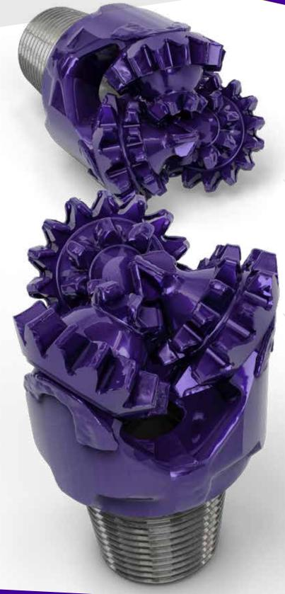
Varel's classic open bearing steel teeth bits for remedial, re-entry, and water well applications. All bits incorporate open throat hydraulics and can accommodate either regular through string flow or reverse circulation which is frequently used to re-enter wells. L2, L1, and LH1 are offered from softest to hardest of the cutting structure applications.
